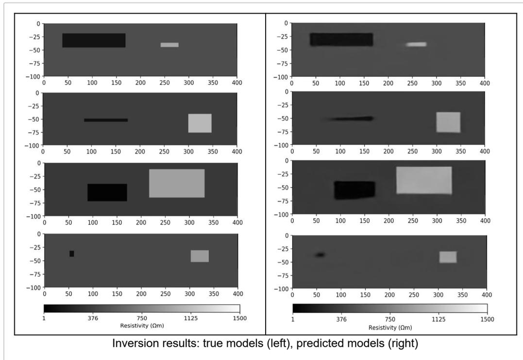
The results confirm the efficacy and effectiveness of the proposed U-Net architecture in solving the 2-D ERT inverse problem for subsurface resistivity modelling.
