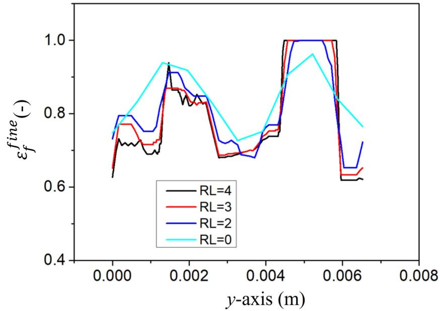
Figure 10: Variation in  $\varepsilon_f^{fine}$  for successive slices in the x-z plane along a straight line parallel to the  $y$ -axis (as indicated in 8) for three different mesh refinement levels ( $RLs$ )
