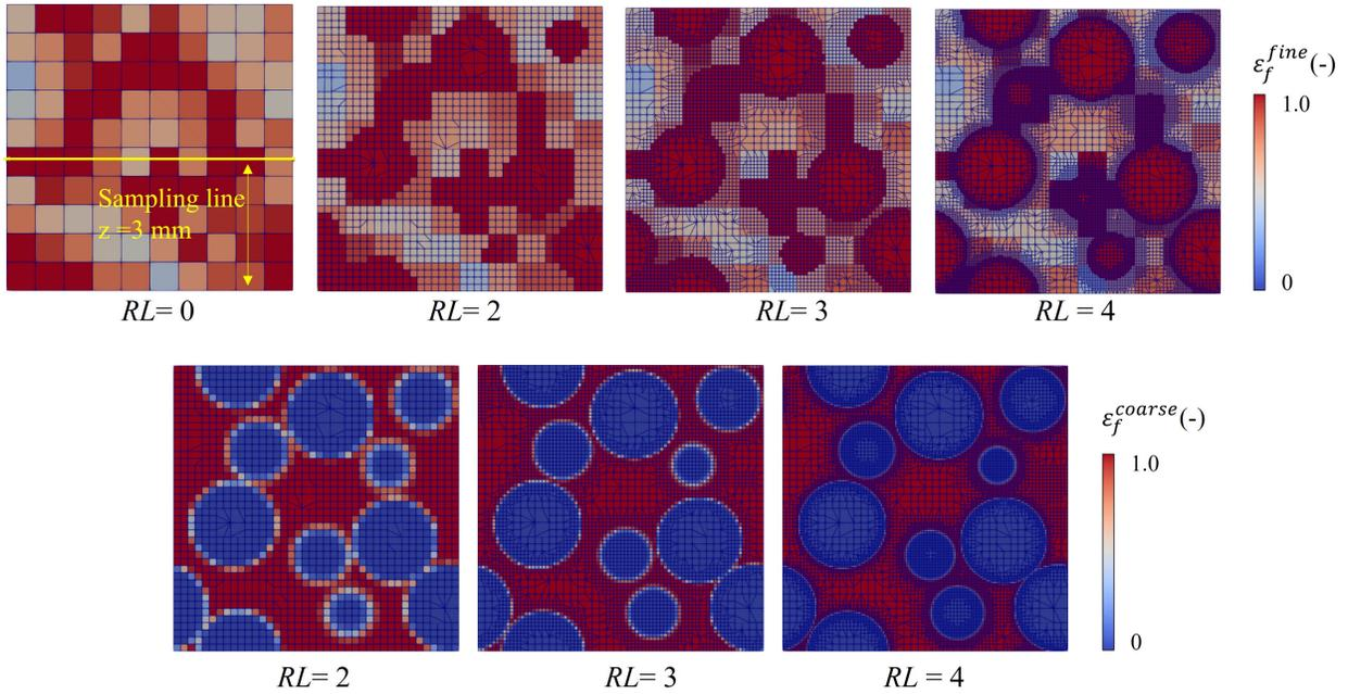
Figure 8:  $\varepsilon_f^{coarse}$  and  $\varepsilon_f^{fine}$  fields under different mesh refinement levels (the slice was taken in the  $y$ - $z$  plane at a distance of 0.33 cm from the inlet, the size ratio of particles in the sample is 4)
