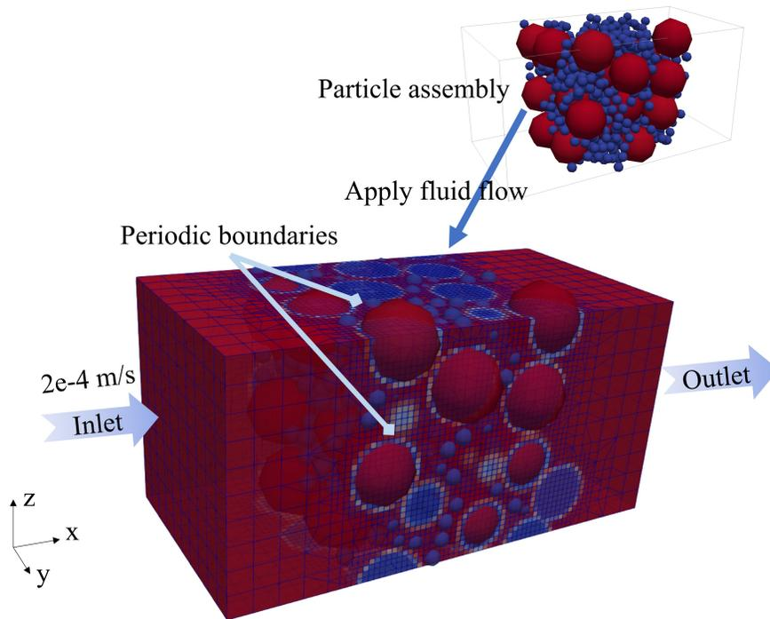
Figure 4: Illustration of particle assembly considered (with a coarse-fine particle size ratio of 4) including annotation of boundary conditions
