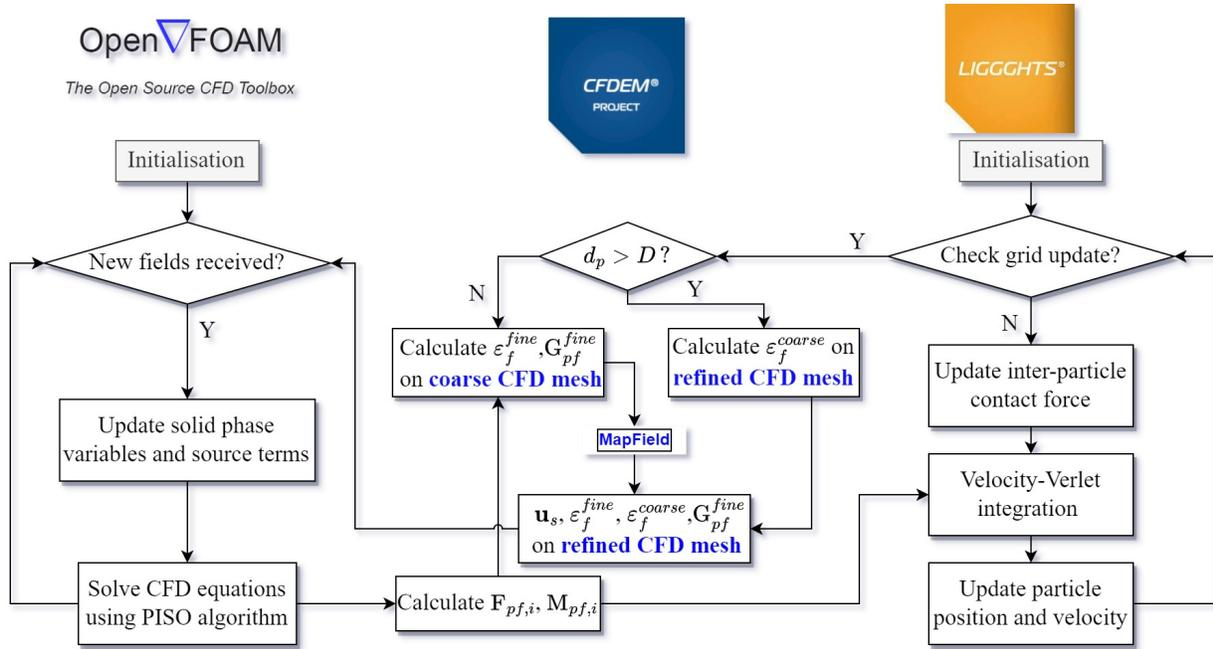
Figure 3: Flowchart of the two-grid semi-resolved CFD-DEM
