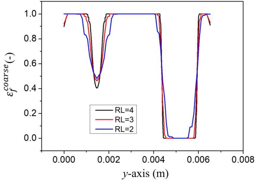
Figure 9: Variation in  $\varepsilon_f^{coarse}$  for successive slices in the x-z plane along a straight line parallel to the  $y$ -axis (as indicated in 8) for three different mesh refinement levels ( $RLs$ )
