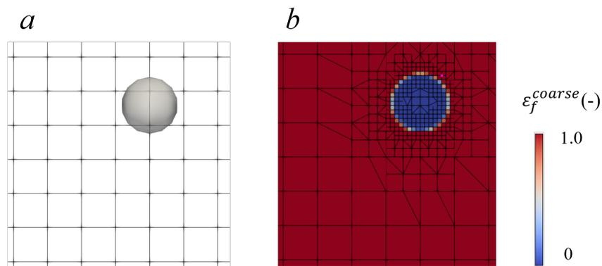
Figure 2: Schematic diagram of the mesh refinement (a) coarse mesh (b) refined system with a mesh refinement level of 3
