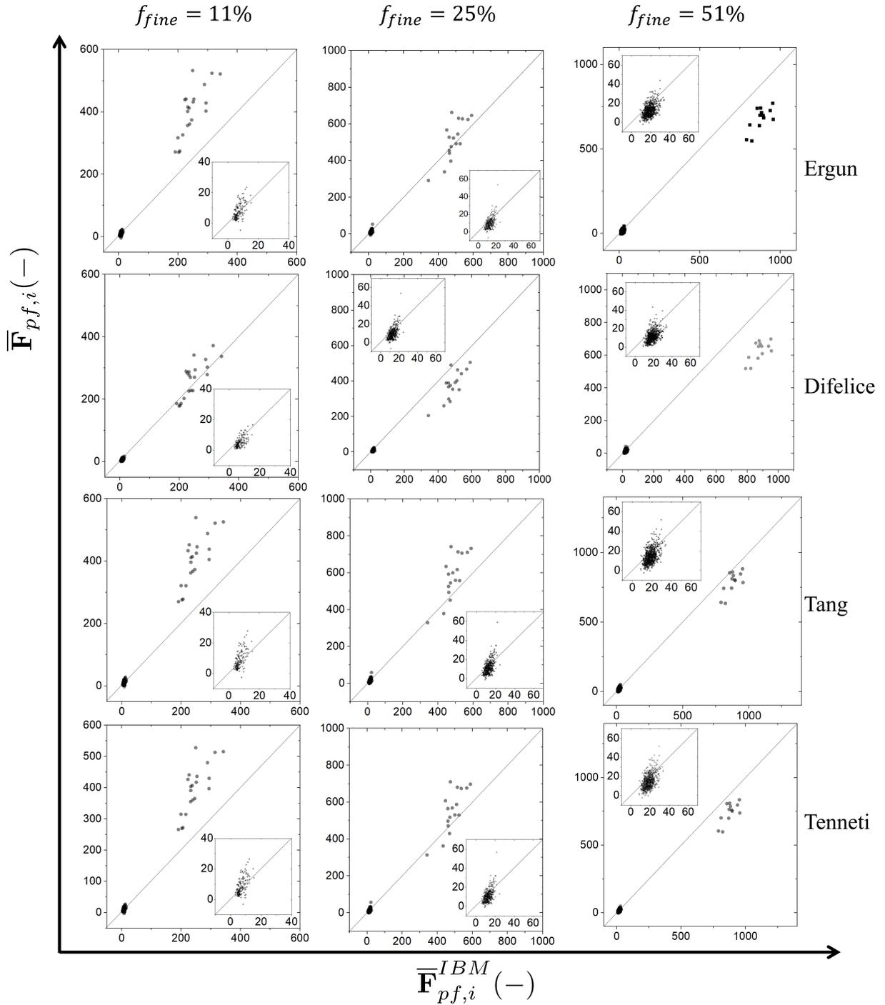
Figure 13: Comparison of the  $\mathbf{F}_{pf,i}$  from fully resolved and semi-resolved solvers illustrating sensitivity to the drag model adopted for the finer particles (inset gives magnified image of data for the finer particles)
