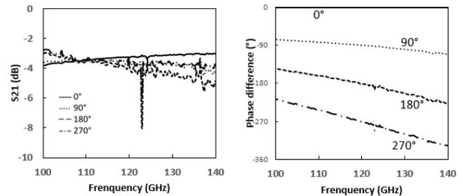
**Fig. 6** 2-bit RTPS results after optimization with flipped PIN diodes
