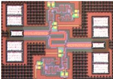
**Fig. 3** Chip microphotograph of 2-bit RTPS
