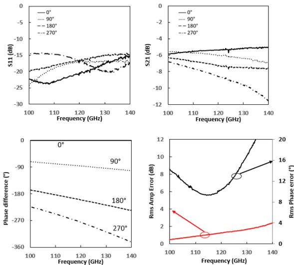
**Fig. 4** 2-bit RTPS measurement results with PIN diodes modelled by resistance or capacitance.
