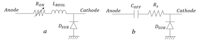
**Fig. 5** PIN diode electrical model
