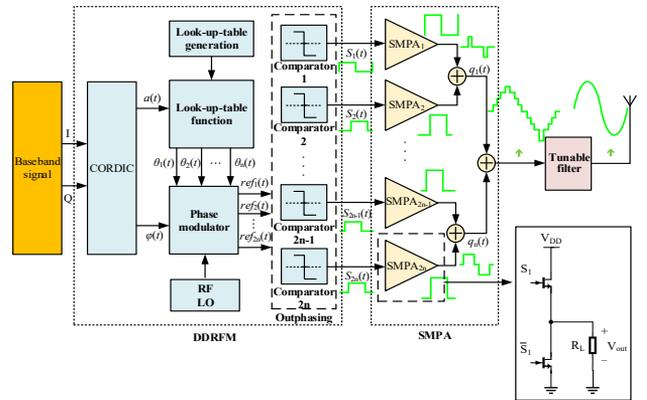
Fig 4 Structure of RF-PWM based ADTx with half-bridge SMPA chip
