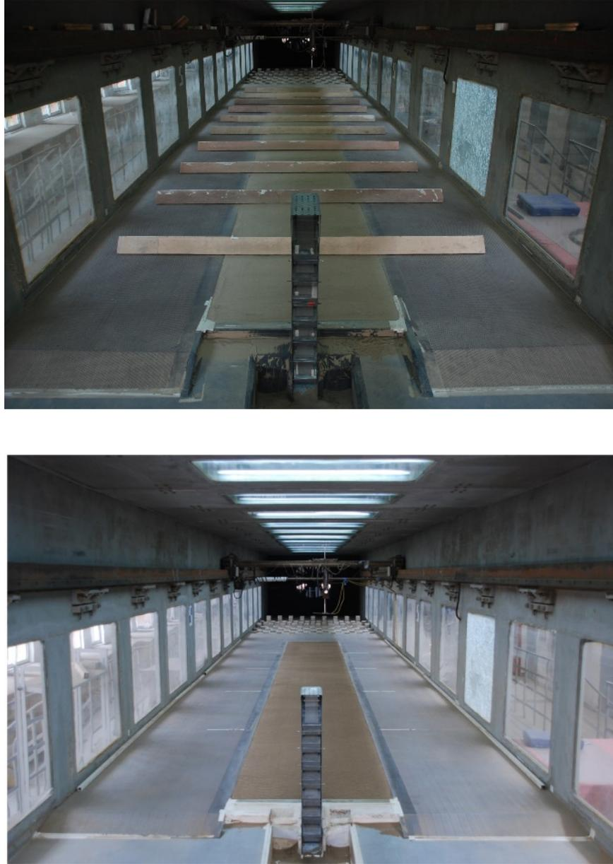
**Fig. 2** Ridges arrangement in the wind erosion experiments. This figure shows ridge height is 10 cm and spacing is 10H (a) and one with no ridges condition (b).
