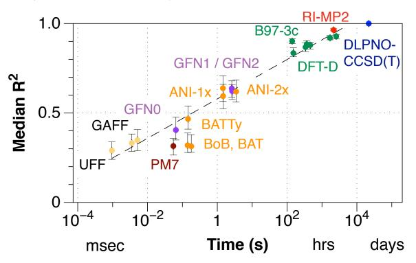
Figure 3: Comparison of single-core computational time required for energy evaluation (in log scale) to median  $R^2$  found when compared to DLPNO-CCSD(T) energies. Error bars indicate 95% confidence intervals of time and median  $R^2$  from bootstrap sampling. Dashed line indicates approximate "best current method" threshold defined from force fields through RI-MP2 methods.
