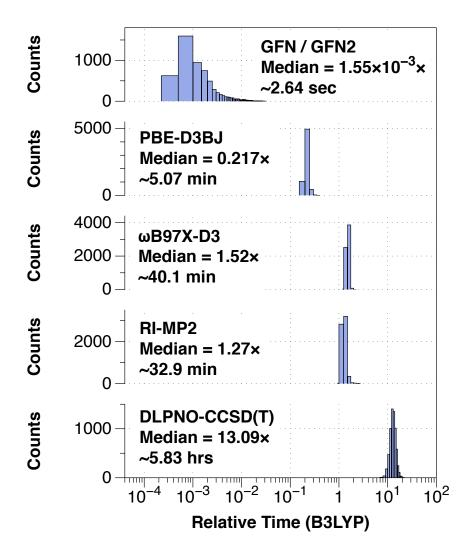
Figure 2: Histograms of relative timings for key methods considered, normalized to B3LYP-D3BJ single points on the same molecule, using ORCA 4.0.1. Median relative times and median wall clock times for single-core runs are included for reference.
