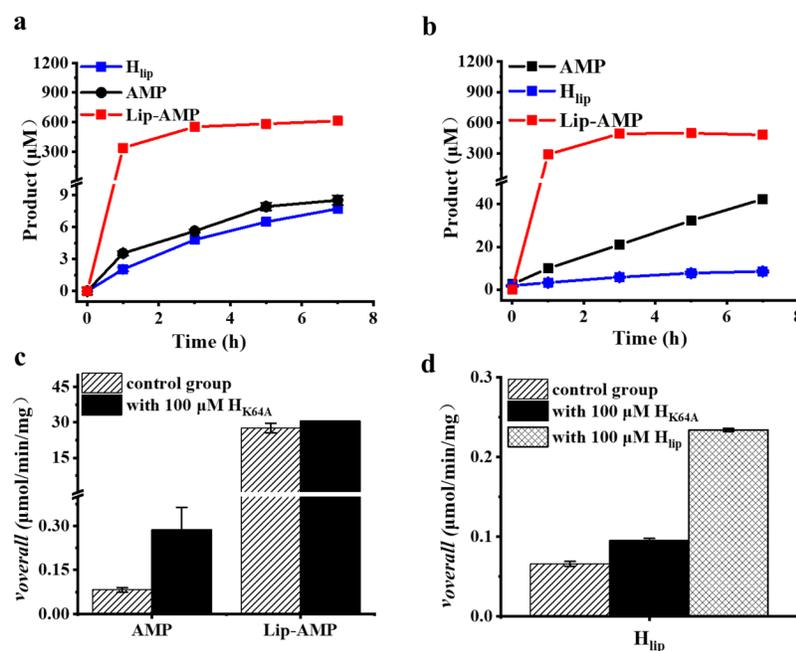
**Figure 4.** Time course of the formation and the specific formation rates of Lip-AMP, AMP and H<sub>lip</sub> in the overall reaction: (a) in a normal assay with 10 µM H<sub>apo</sub> without addition of H<sub>K64A</sub>; (b) with the addition of 100 µM H<sub>K64A</sub>. (c) the specific formation rates of Lip-AMP and AMP; (d) the specific formation rates of H<sub>lip</sub>.
