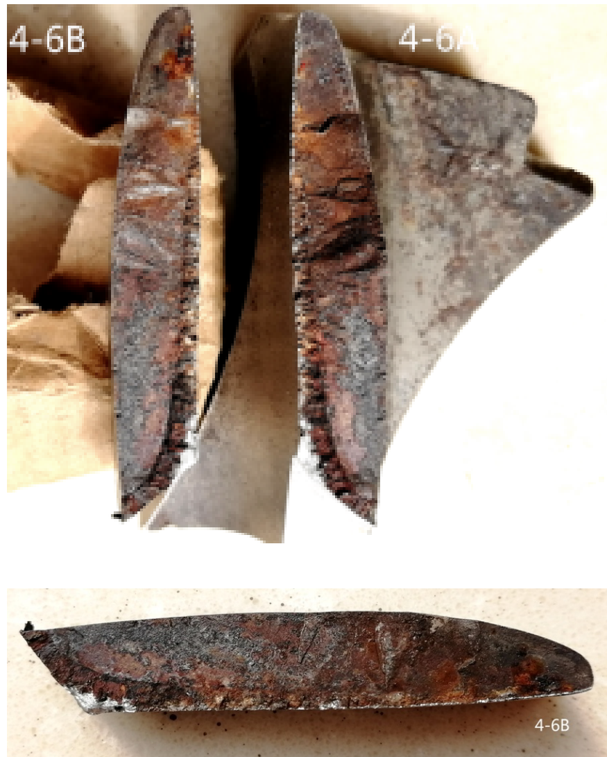
Fig. 10 Original surface not cleaned (after fracture opening)
