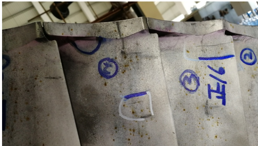
Fig. 3 Water erosion of last stage blade
