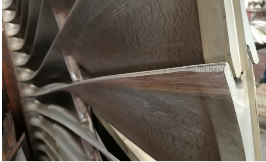
Fig. 3 Water erosion of last stage blade
