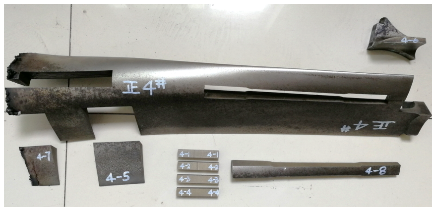
Fig. 5 Sampling(among them, 4-5 is the element analysis sample, 4-6 is the metallographic sample, 4-8 is the tensile sample, 4-1, 4-2, 4-3, 4-4 is the impact sample)
