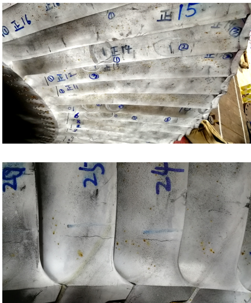
Fig. 4 A:Cracks on the top of blade,B:Cracks in the middle of blade,C:Cracks at blade root
