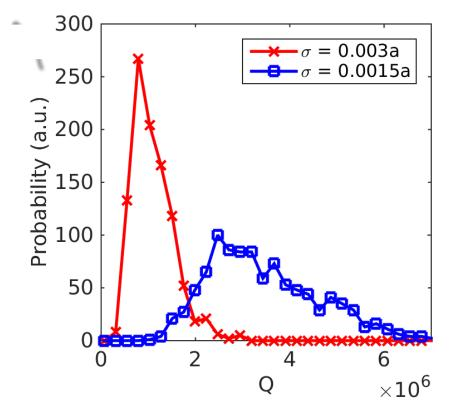
Figure 2: Histograms of the probability distribution of the quality factor  $Q_e$  in presence of disorder for the optimized 8-shift cavity. 1000 disorder realizations were computed using the GME.
