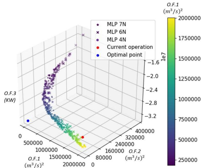
**Figure 15.** Pareto front for models with MLP and NSGAI optimizers.
