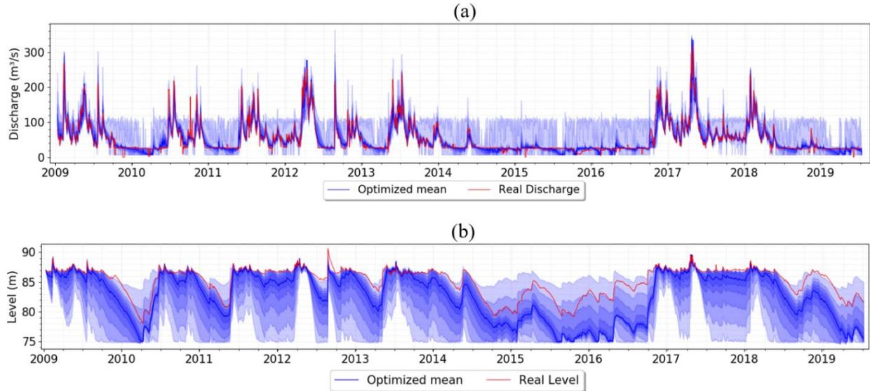
**Figure 12.** Envelope for hydrographs generated by all reservoir operations obtained from optimization. (a) flow rates and (b) levels. The mean values of the reservoir operations for the entire population are shown in dark blue, and the gradient color shows the quintiles.
