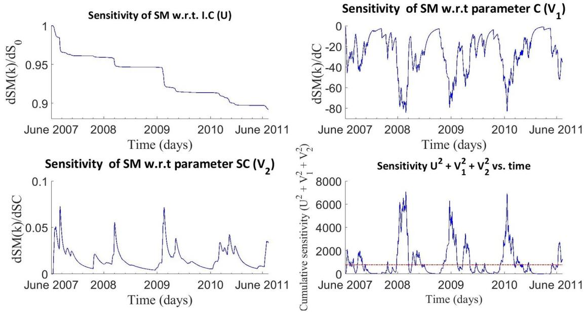
Figure 4: Sensitivity evolution of the soil moisture with respect to a) Initial condition ' $S_0$ ', b) parameter 'C', c) Parameter 'SC', and d) cumulative sensitivity.
