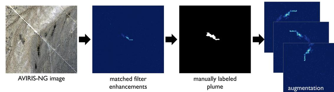
Figure 2. Preprocessing steps before feeding the data into U-Net.
