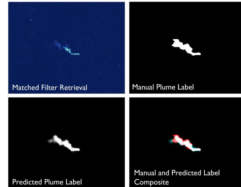
Figure 3. Methane plume images from flight-line ang20180917t213701
