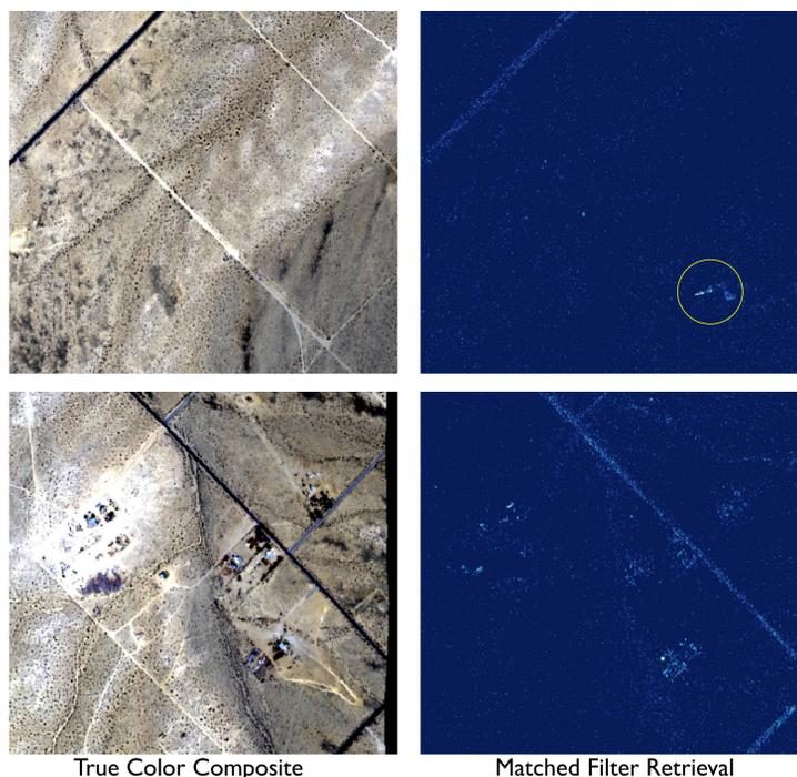
Figure 1. True color composites and matched filter retrievals of the 2018 time series data. In addition to finding the plume in the top-right tile (yellow circle), the matched filter also identified a variety of roads, roofs, and small portions of desert as false methane enhancements.
