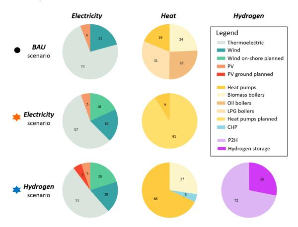
Energy production share (%) of different technologies for different energy carriers. BAU scenario solution is compared with the optimal *Electricity* scenario and *Hydrogen* scenario solutions characterized by a CO<sub>2</sub> cost of 50 €/ton.
