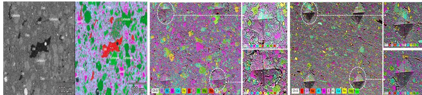
Left: (BSE) micrograph (left) and the EDS map (right) obtained from a polished surface of Caney sample. Middle: BSED surface chemistry at 20 kV of the Sample A(Brittle). Right: BSED surface chemistry at 20 kV of the Sample B(Ductile) where indentation was done. Abundant magenta (quartz) with lesser amounts of olive green (dolomite) and pale blue (calcite). Yellow is pyrite, whereas clay minerals make up most of the fine grained matrix.
