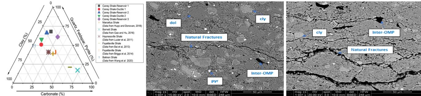
Left: Mineralogy of the Caney Shale compared to other formations; Middle: SEM photo micro graph depicting Sample A(Brittle); Right: SEM photomicrograph, Sample B(Ductile) showing clays, fractures,and organic matter.
