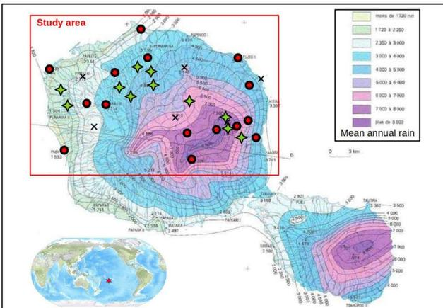
Figure 1: Temporary densification (green diamonds) of the long term rain gauge network of northern Tahiti Nui (red dots: active gauges, black crosses: malfunctioning gauges). Background rain map from: Lafforgue (1993), Atlas de la Polynésie.
