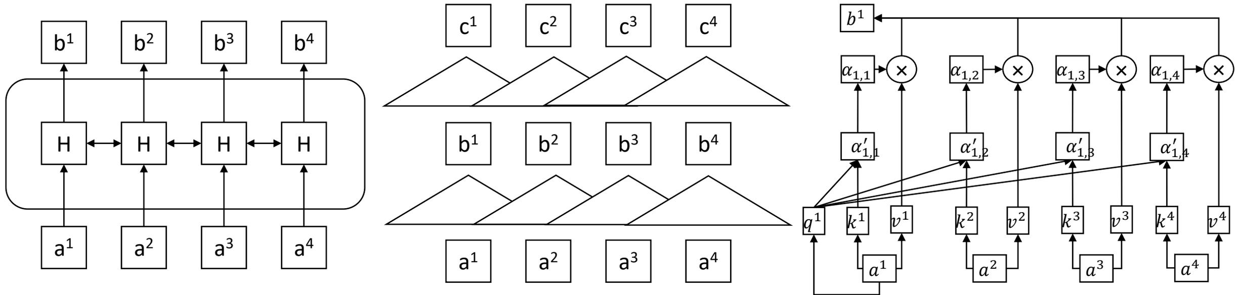
Figure: LSTM, TCNN and Attention model architecture.
