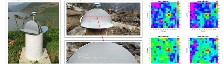
Fig. 7 Tested dihedral corner reflectors and its intensity in the test filed.
