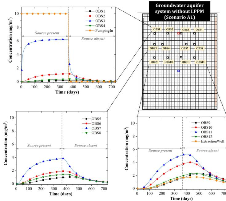
Figure 6: Breakthrough curves(BTCs) predicted at various observation wells
