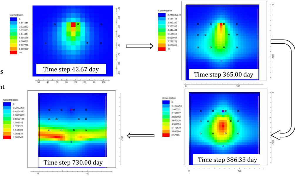
Figure 5: Contaminant plume evolution in the homogeneous aquifer system up to 730 days time level
