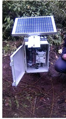
Left: First generation station. Stations suffered water infiltration, vandalism (pictured), and power outages.
