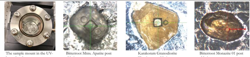
The sample mount in the UV-laser chamber. Bitterroot Mtns. Apatite post-ablation. Karakoram Granodiorite Titanite post-ablation. Bitterroot Monazite 01 post-ablation.
