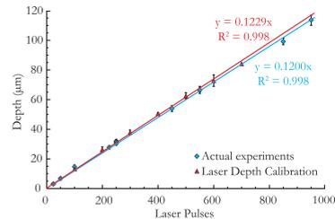
Drill rate calibration for a 100 µm round spot in Durango apatite compared to pit depths from actual LADP experiments. Drill rates are mineral and spot size specific. The depth calibration is linear to depths of >100 µm.
