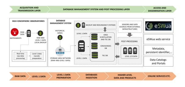
In the "acquisition layer" the raw observations are real-time processed at the remote facilities to produce Level 1 ionospheric data in different encoding formats, depending on the particular acquisition instrument. A copy of the raw-data is locally stored while the Level-1 data (and the raw data when possible) are transmitted in near real-time to the INGV central repository in Rome.
