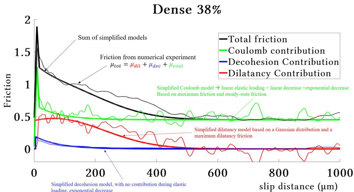
**Figure 12.** Friction-slip curve with different contributions (dilatancy in red, Coulomb in green and decohesion in blue) - dense sample - 38% of cohesion - The black curve is the sum of all contributions. Bold lines represent the proposed simplified model and thin curves the numerical results.
