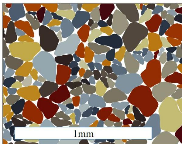
**Figure 2.** Grains sample generated with Packing2D (Mollon *et al.*, 2012). Angular shape and fractal distribution ( $D=2.6$ ).
