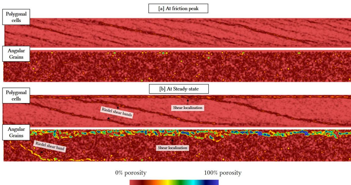
**Figure 10.** Fracture patterns in dense third body layers as a function of the percentage of porosity within the sample for angular grains (i.e. 11% initial porosity) and polygonal cells (i.e. 0.01% porosity) – [a] Friction peak [b] Steady-state
