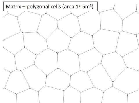
New gouge sample with Polygonal cells (i.e. 0.01% porosity) and Coulomb friction law (no cohesion)
