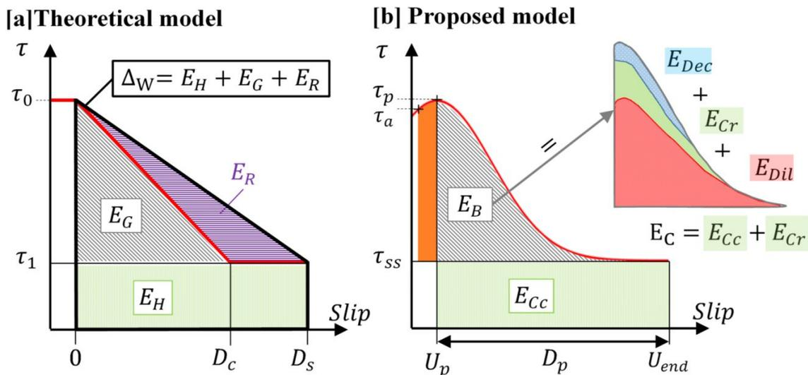
**Figure 14:** (a) Theoretical model of energy budget  $\Delta W$  as the sum of a fracture energy  $E_G$ , a radiated energy  $E_R$  (propagating by the mean of elastic waves) and a frictional energy  $E_H$  (dissipated within the slip zone).  $\tau_0$  is the initial static shear stress,  $\tau_1$  the dynamic shear stress,  $D_c$  is the slip
