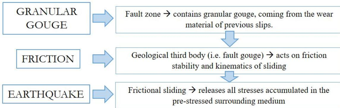
The aim is to link third body properties to its rheological behavior in order to access information on slip triggering.
