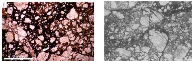
**Figure 1.** Images from (Muto *et al.*, 2015), (Blenkinsop, 1991) with granular and faceted grain shape
