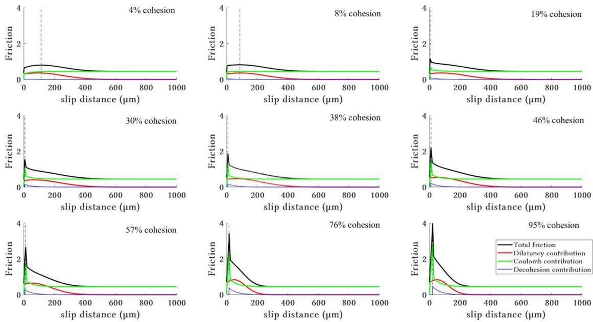
**Figure 13.** Proposed simplified models - Evolution of friction contributions as a function of the slip distance, for different percentage of cohesion. Dense sample - Mildly cohesive regimes with a diminution of the pre-peak phase with the increase of cohesion (0% to 25%) – Cohesive regimes with a negligible pre-peak phase but an important influence of friction peak (25% to 75%) – Ultra cohesive regimes with almost not pre-peak phase and an very high Coulomb friction peak (75% to 100%).
