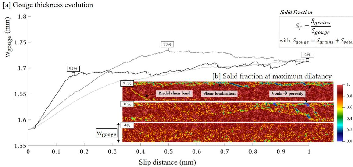
**Figure 8.** [a] Gouge thickness evolution (mm) as a function of the slip distance (mm) for 4%, 38% & 95% of cohesion – [b] Solid fraction at the maximum dilatancy observed in the three samples, presence of Riedel bands and shear localization.
