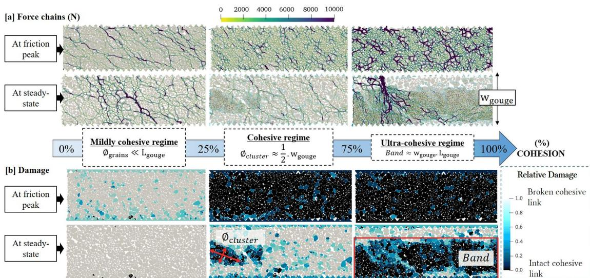
**Figure 9.** [a] Force chains as a function of the percentage of cohesion, at friction peak and at steady state. Three regimes of cohesion. [b] Relative damage snapshot for 4%, 38% & 95% of cohesion for dense samples. This damage is set to 0 when cohesive bonds are first established (all the bonds are intact) and may evolve until 1 if all these bonds reach the “broken” status.
