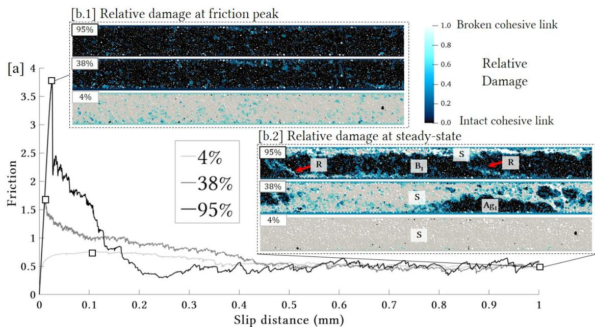
**Figure 7.** [a] Friction coefficient as a function of the slip distance of the upper rock wall (mm) [b] Relative damage snapshot for 4%, 38% & 95% of cohesion in the dense sample (entire granular gouge). This damage is set to 0 when cohesive bonds are first established (all the bonds are intact) and may evolve until 1 if all these bonds reach the “broken” status. R represent the Riedel shear bands and S the horizontal shear localization.
