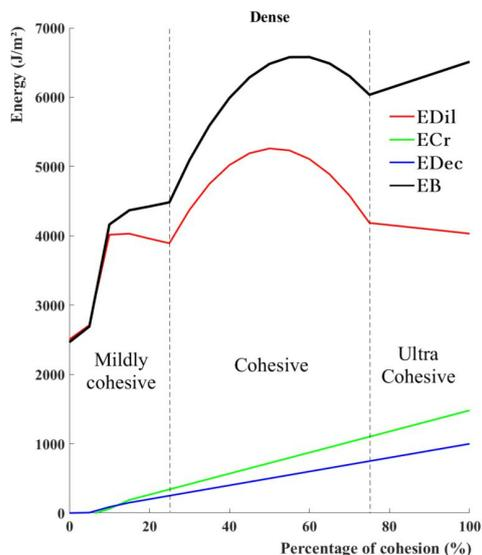
**Figure 15.** Breakdown energy ( $J/m^2$ ) coming from the different contributions as a function of the percentage of cohesion within the gouge for dense samples.  $E_B$  (in black) gathers a dilatancy energy  $E_{dil}$  (in red) linked to sample dilation (mechanical energy), a Decohesion energy  $E_{Dec}$  (in blue) coming from the breakage of cohesive links (surface creation energy) and  $E_{Cr}$  (in green), a part of Coulomb energy  $E_C$ .
