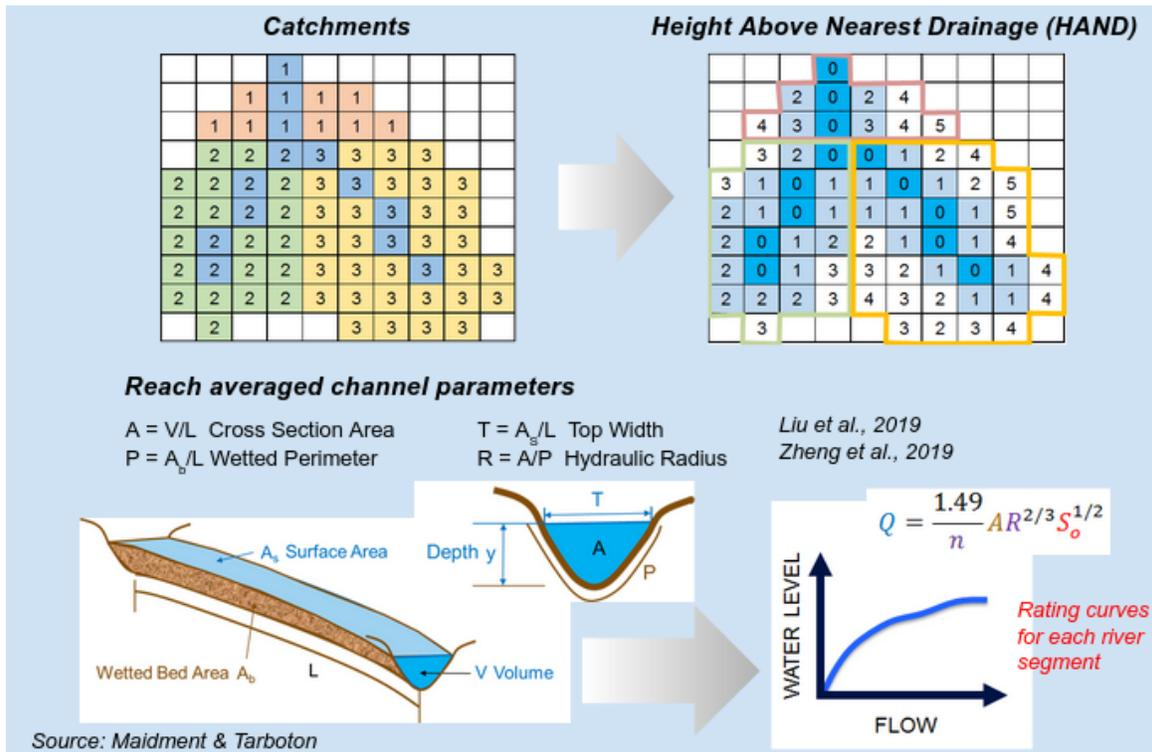
**Figure 2:** Demonstrates delineated stream reaches and catchments as well as relative elevation values known as HAND. Reached averaged channel parameters are sampled from HAND raster and inputted to Manning's equation to establish stage-discharge relationship.
