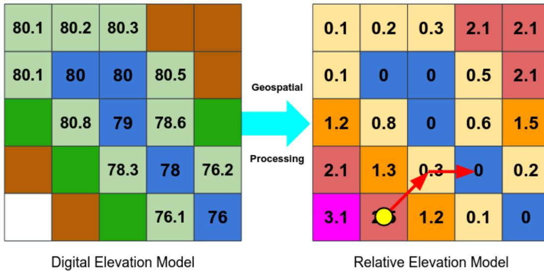
**Figure 1:** Demonstrates conversion of digital elevation model (DEM) referenced to mean sea level to relative elevation model (REM), also known as HAND, referenced to local, relevant river channel elevations.
