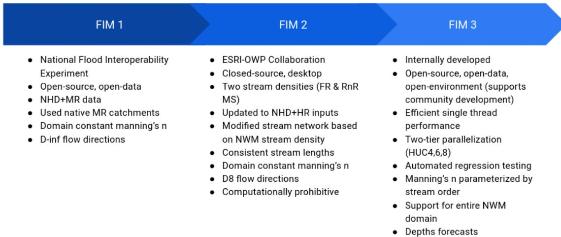
**Figure 3:** OWP FIM is based on the HAND method<sup>2</sup> originally implemented by the National Flood Interoperability Experiment (NFIE). Details the evolution of the technology and capabilities.
