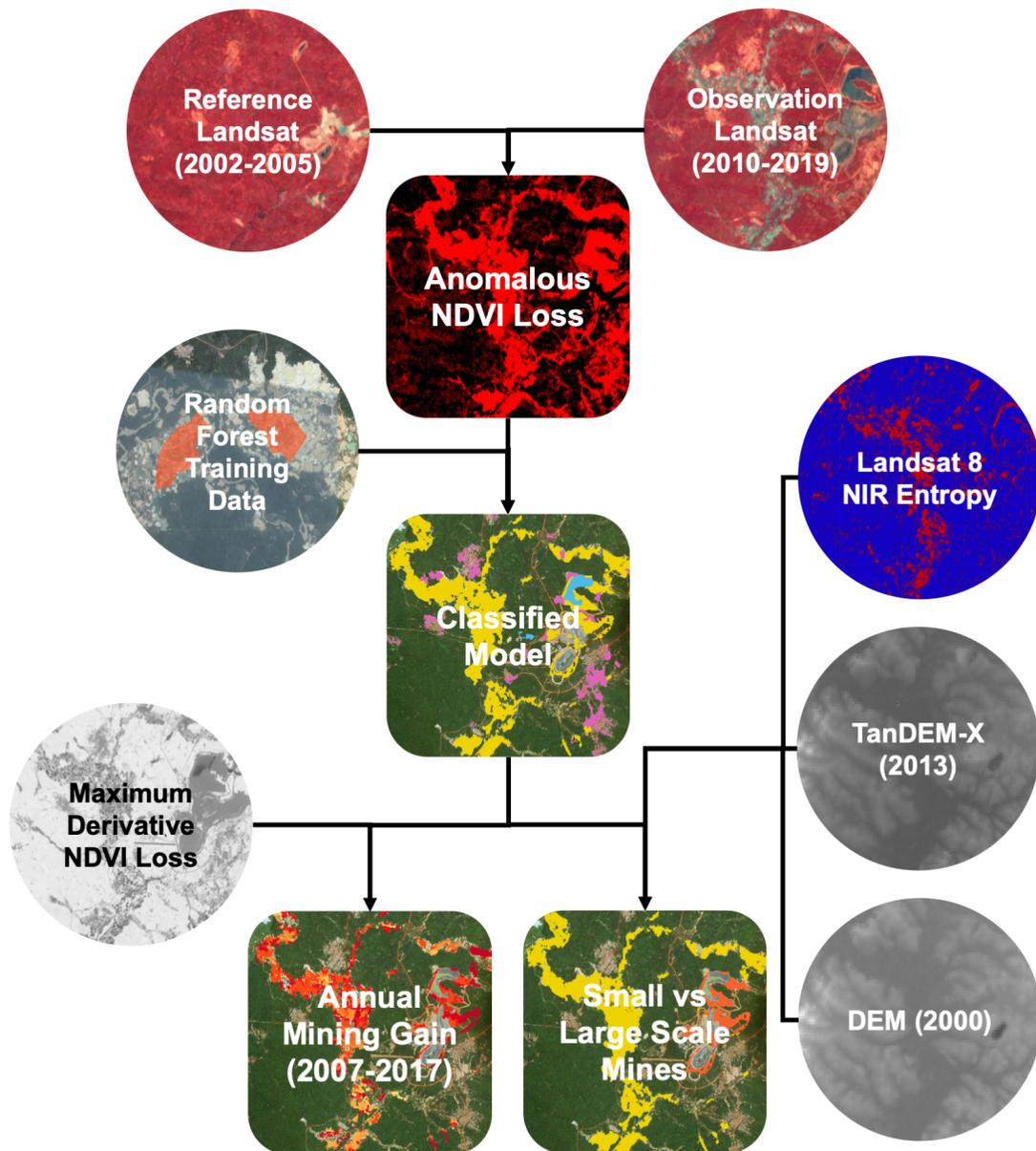
NDVI change anomalies were detected using historical Landsat 5 TM, 7 ETM+, and 8 OLI image collections. An imagery timestack for 2010-2019 was compared to a reference period of 2002-2005. A mean NDVI loss of 0.15 or more was considered as substantial and prolonged disturbance. A random forest classification was used to classify these loss areas as Mining, Urban, Water, or Other loss. Large scale mines were separated from artisanal mines with an additional random forest classification.
