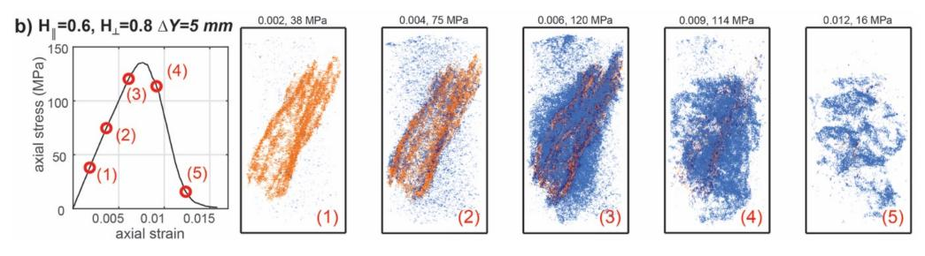
Below: Surprisingly, the tested combinations of Hurst exponents (b) and roughness amplitudes (c) *do not produce changes* in the macroscopic strength that are larger than those produced by random variations in particle packing (d).
