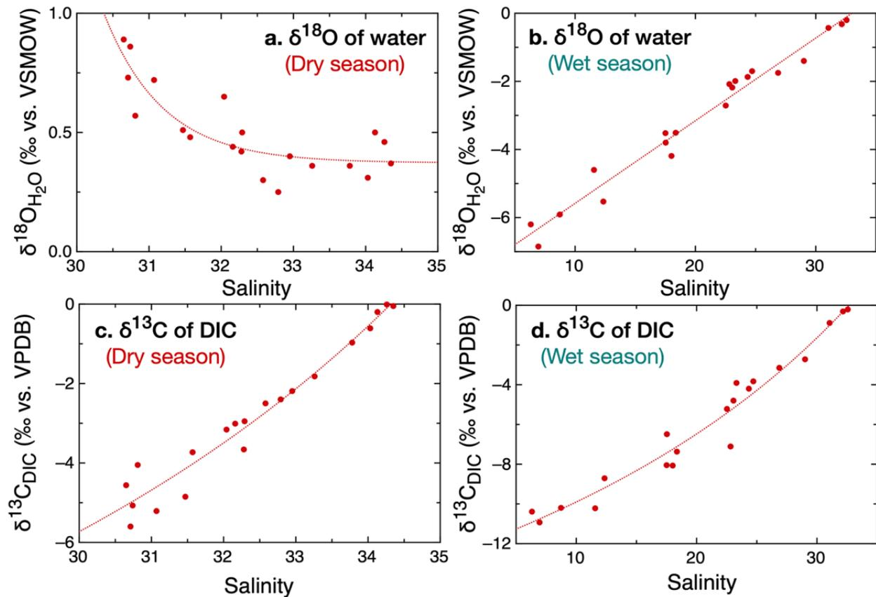
Figure 3. Relationships between the salinity and the  $\delta^{18}\text{O}$  of water (*top*) and the  $\delta^{13}\text{C}$  of DIC (*bottom*) in the dry (*left*) and wet (*right*) seasons in the surface water of Batan Bay. Freshwater-endmember  $\delta^{13}\text{C}_{\text{DIC}}$  was evaluated by the conservative mixing model as  $-16.2\text{‰}$  and  $-12.5\text{‰}$  for the dry and wet seasons, respectively.
