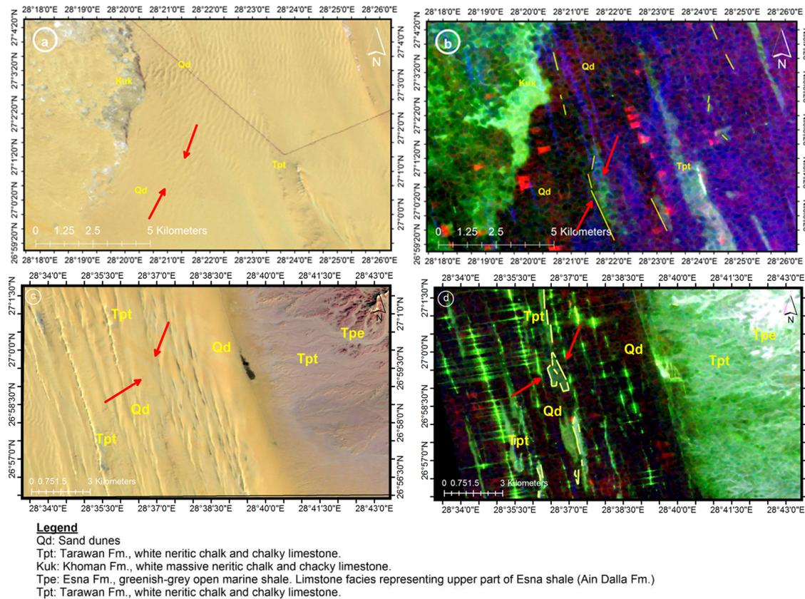
Initially, Full polarimetric images are represented in Pauli RGB, then, the interpreted features in the two areas of interest, The buried subsurface features exist in radar images, while remain unobserved in optical image. The distribution of subsurface features are strongly linked with backscattering coefficient.
