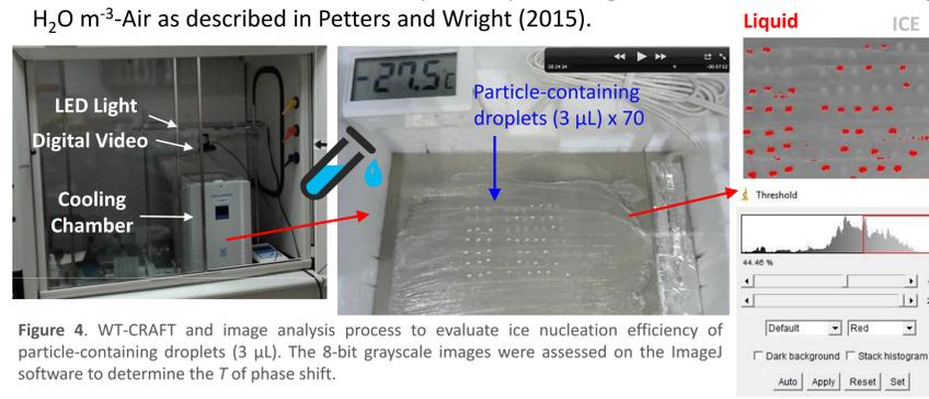
Figure 4. WT-CRAFT and image analysis process to evaluate ice nucleation efficiency of particle-containing droplets (3  $\mu$ L). The 8-bit grayscale images were assessed on the ImageJ software to determine the  $T$  of phase shift.
