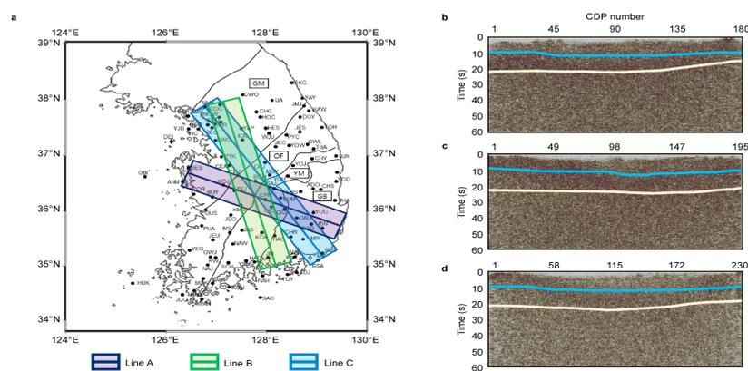
**Fig. 1.** Map showing the study area of the Korean peninsula (a) and seismic reflection images of the three profile lines (b-d); (b) Line A, (c) Line B, and (d) Line C. Note that the light-blue line and beige line indicate the Moho (at 9-12 s) and LAB horizons (at 17-23 s), respectively.
