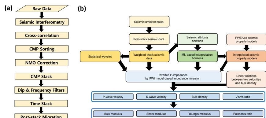
**Fig. 2.** The workflow of seismic data processing (a), and seismic inversion strategy (b) by using the seismic data and seismic models from the FWEA18 datasets.
