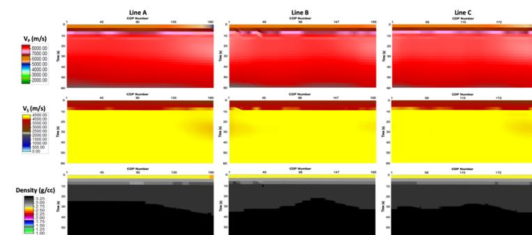
**Fig. 4.** Initial seismic velocity and density models for the background models of the model-based impedance inversion. Note that these are developed by interpolation of the original sparse FWEA18 model based on the seismic data acquisition geometry.
