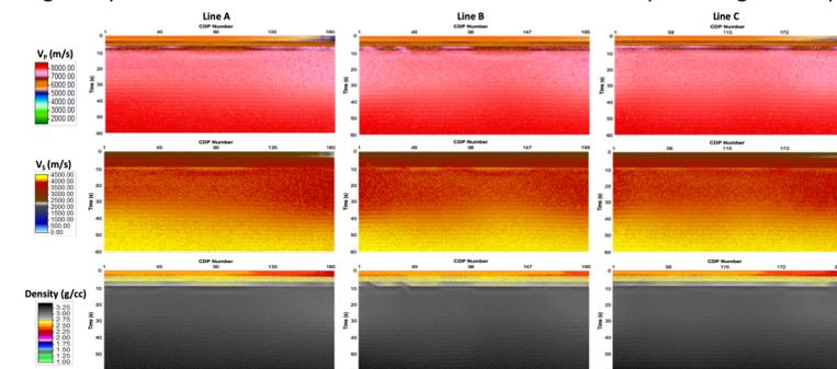
**Fig. 5.** Inverted seismic velocity and density models from the initial models (Fig. 4.) and the post-stack seismic data. Through the linear relationships of Vp-Vs-density in the FWEA18 research, we can estimate the Vp, Vs, and density variations from the inverted impedance model.
