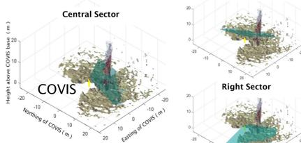
COVIS operates alternately in Imaging and Diffuse-flow modes for imaging and mapping of hydrothermal discharge from focused and diffuse sources, respectively
