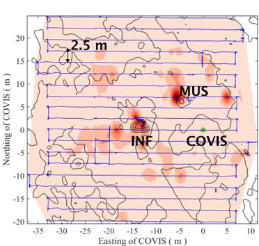
Near-bottom temperature within ASHES was surveyed using a 5-m thermistor array hanging beneath an ROV in Jun 2018. INF: Inferno vent MUS: Mushroom vent
