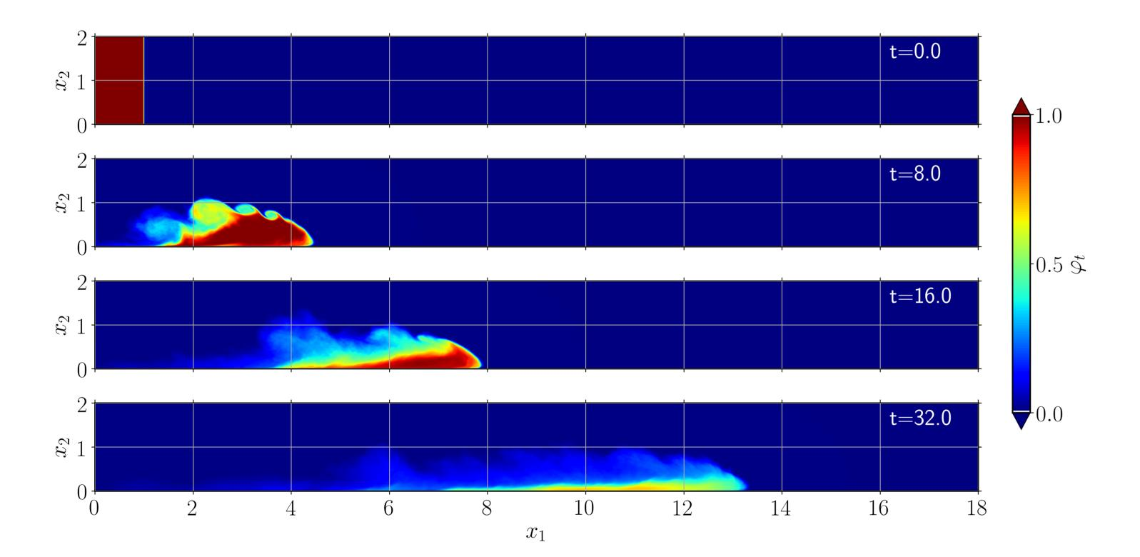
Figure 1:Flow evolution, represented by the spanwise-averaged total concentration field. Spanwise extension is  $L_3 = 2$ . The computational domain is discretized in  $1153 \times 257 \times 121$  mesh nodes, and a time step of  $1.2 \times 10^{-3}$  is used for a total of  $8 \times 10^4$  iterations.
