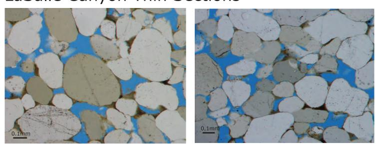
Thin sections of rock from Illinois Canyon displayed greater porosity and less cement than rock from LaSalle Canyon. Measurements of rock strength taken with a Schmidt hammer indicated slightly weaker rocks in Illinois Canyon. Erosion estimates from SfM indicated that the Illinois Canyon surface eroded more than the LaSalle Canyon surface.
