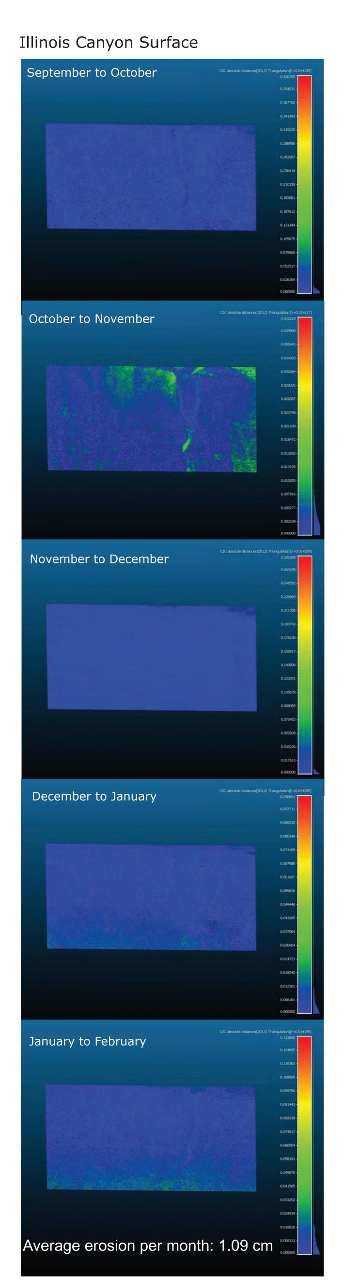
The photogrammetric SfM analysis detected measurable change on a centimeter to millimeter scale. Changes along footpaths were observed when visitor traffic was high. During winter months when visitor traffic decreased, rainfall and snowmelt primarily caused mobilization and removal of loose sediments covering bedrock surfaces.
