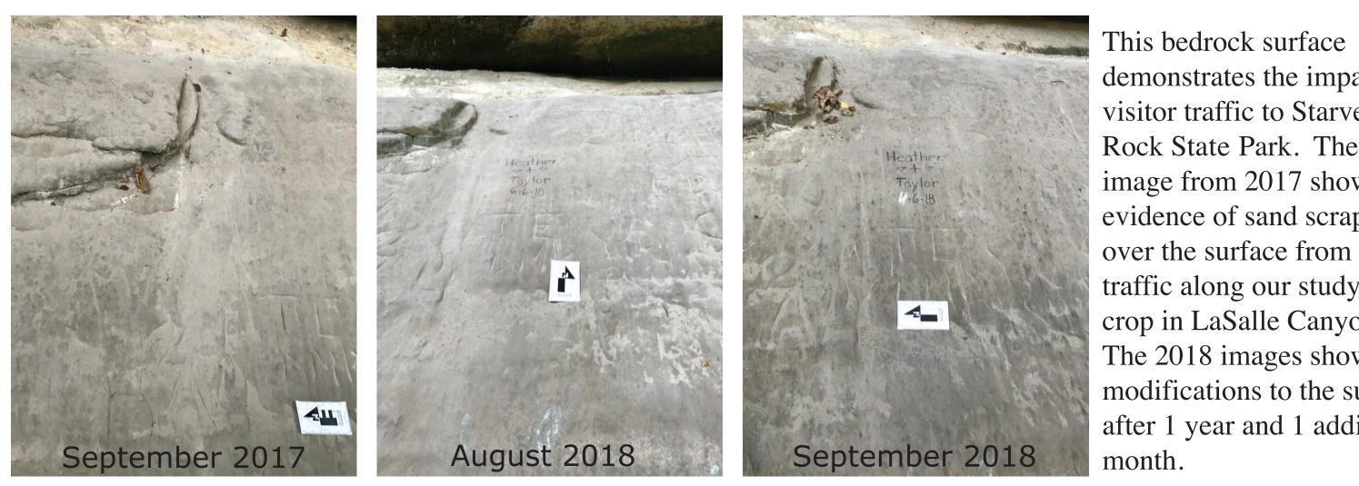
The St. Peter Sandstone is a weakly cemented, extremely friable quartz arenite, making it susceptible to human disturbance and rapid natural erosion. This study explores how quickly present day changes occur along bedrock surfaces using photogrammetric Structure-from-Motion (SfM).
