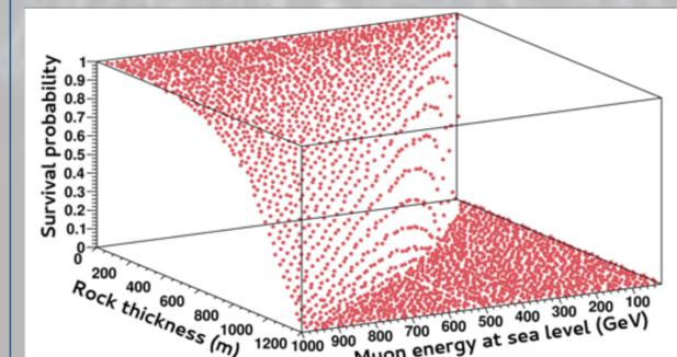
Figure 2.4. Muon survival probabilities as a function of the muon's energy for a standard rock density (2.65 g/cm<sup>3</sup>), from Hivert<sup>[3]</sup>.
