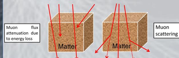
Figure 2.2. (Left) Principle of transmission tomography. (Right) Principle of scattering tomography due to the deviation of the muon.
