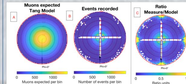
Figure 2.3. Polar chart of the muon arrival distribution according to the Tang model (A), experimental open sky measurement (B) and ratio between them (C).
