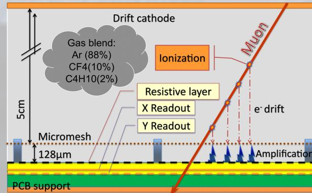
Figure 2.1. Schematic cross-section of the MUST<sup>2</sup> to illustrate its functioning principle.
