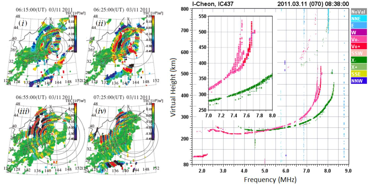
Left: Pattern of concentric TID wavefronts mapped using GPS TEC data recorded over Japan shortly after the 11 March 2011 Tohoku earthquake, reproduced from Tsugawa et al. [2011]. Right: Ionosonde data from I-Cheon, Korea, taken a few hours after the earthquake also show some characteristic signatures of these TIDs, in the form of a Y-forking of the ionogram trace.
