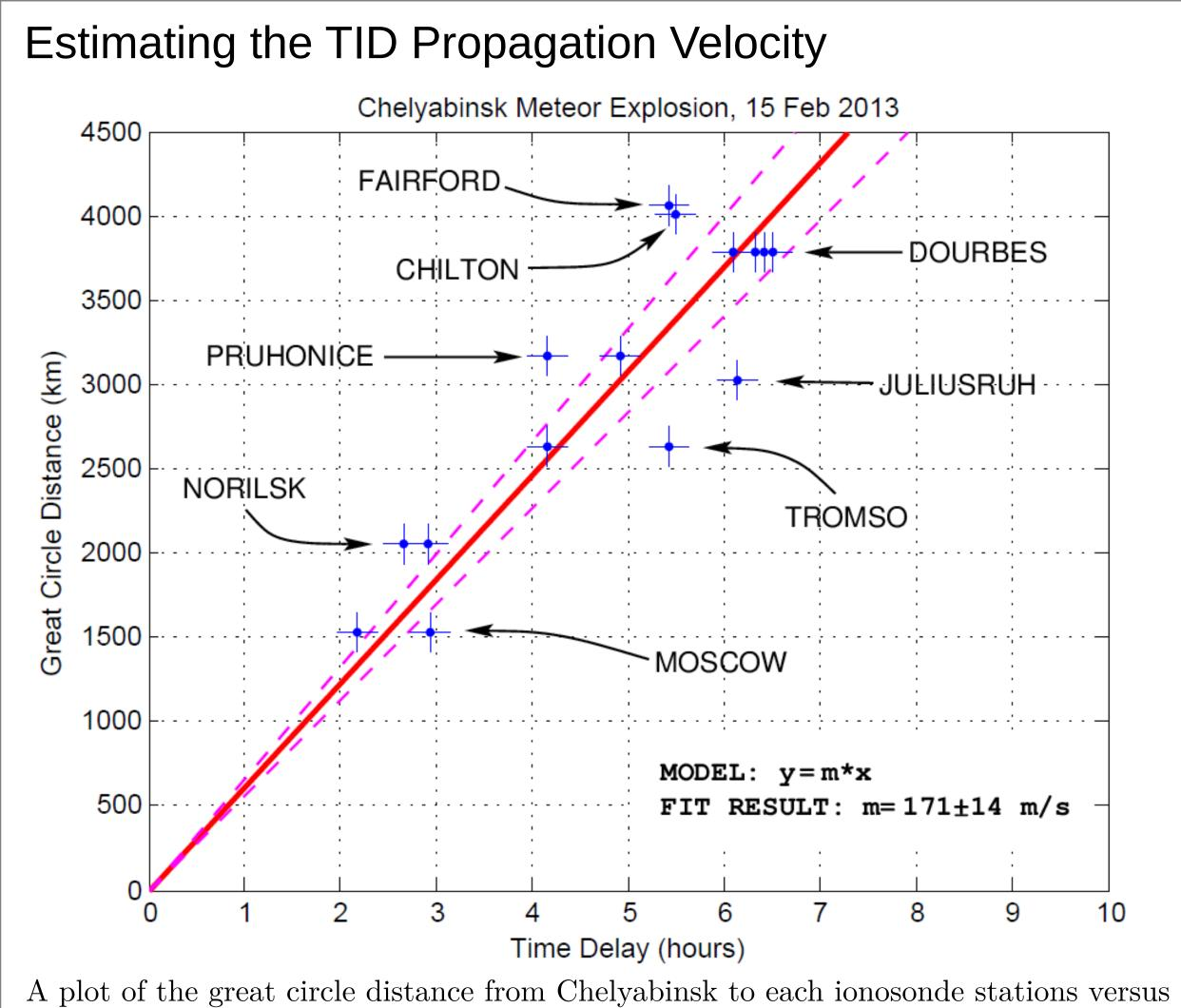
the corresponding time delay for the traveling ionospheric disturbances to arrive. The result of a linear fit to the data points is also overlaid on the graph (solid red line), revealing a propagation speed of roughly 171 m/s. The dashed magenta lines indicate the 95% confidence interval bounds.
