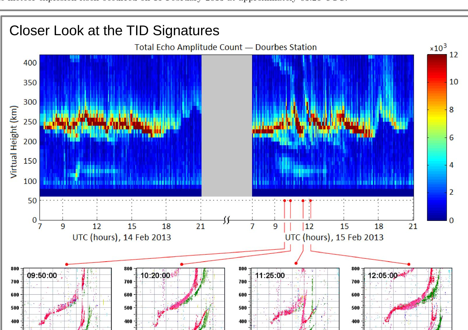
An RTI-style plot of ionogram data from the Dourbes station, covering a representative time window 07:00-21:00 UTC on 14 and 15 February 2013. The colormap indicates the level of the total echo amplitude count at any given virtual height and time, summed over all sounding frequencies. Shown also are samples of individual ionogram at four specific times during the passage of traveling ionospheric disturbances over this station after the Chelyabinsk meteor explosion several hours earlier.
